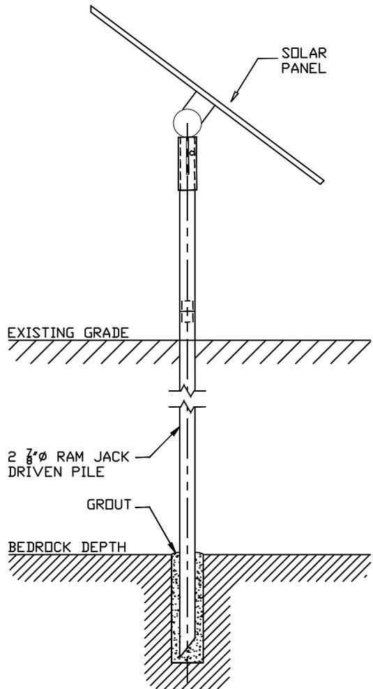
01 TYPICAL PV TRACKER PILE WITH CAP DETAIL
