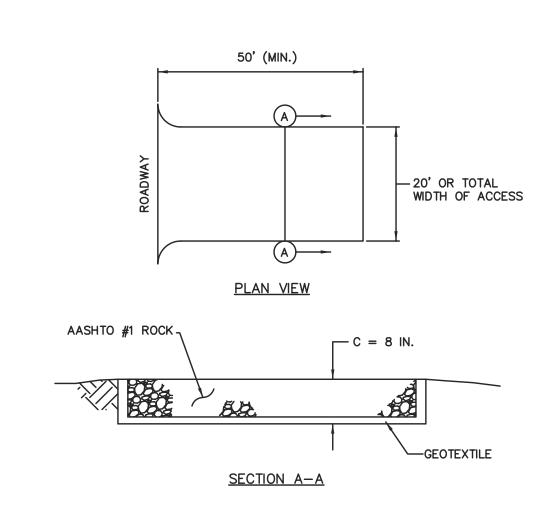
MAINTENANCE: Rock Construction Entrance thickness shall be constantly maintained to the specified dimensions by adding rock. A stockpile shall be maintained on site for this purpose. At the end of each construction day, all sediment deposited on paved roadways shall be removed and returned to the construction site.
