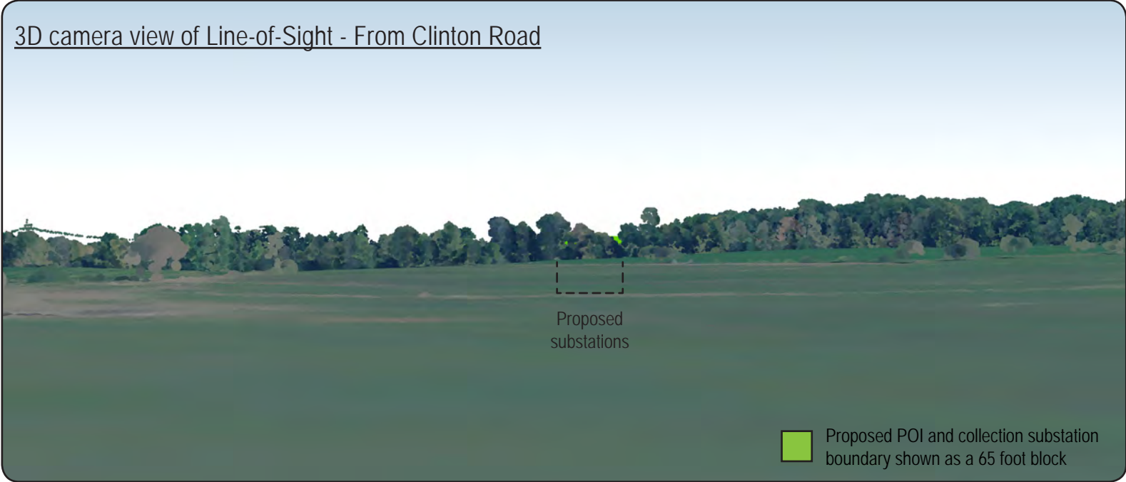
Substation line-of-sight based on lidar data. Vertical scale includes a five times exaggeration.
