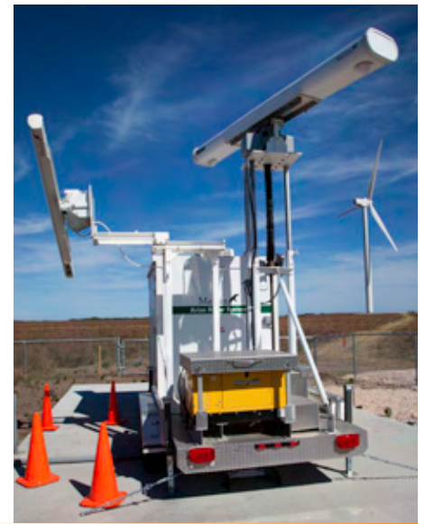
The Merlin Avian Radar System is used to track bird migratory patterns at the Peñascal Wind Power Project in South Texas.
